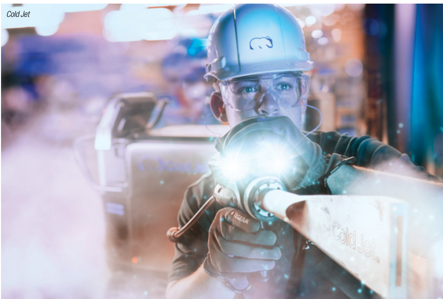
FIGURE 2. Dry ice cleaning uses solid carbon dioxide pellets or microparticles, which are blasted at supersonic speeds and sublime on impact, lifting dirt and contaminants off the underlying substrate. The process is non-abrasive, non-conductive, non-flammable and non-toxic
