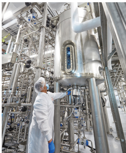
FIGURE 1. Cultured meats are produced in bioreactors (cultivators), such as the one shown here
