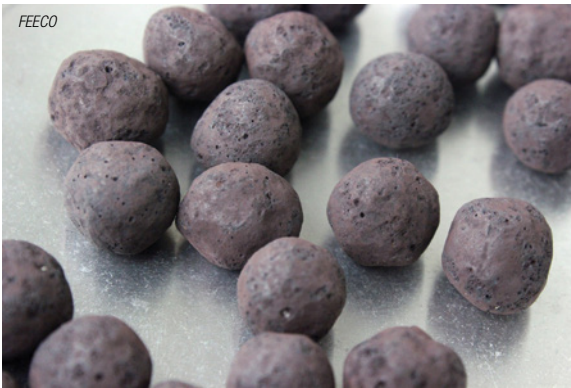
FIGURE 8. When feedstock varies, processors can modify the agitation agglomeration process to maintain product quality
