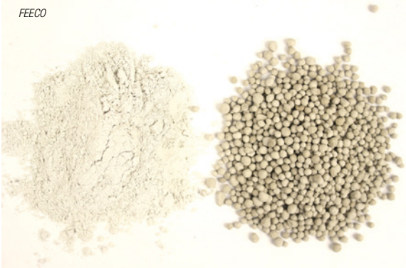
FIGURE 2. Limestone powder (left) can be agglomerated into limestone pellets (right), thereby affecting solids qualities such as flowability, dissolution, particle attrition and more
