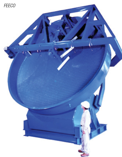
FIGURE 5. This photo depicts a disc pelletizer, showing the rotating disc mounted onto a stationary base
