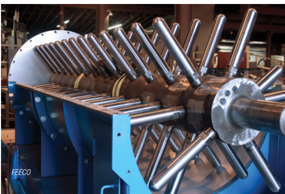
FIGURE 3. Pin mixers, like the one shown here, have a shaft fitted with rods that rotates within a trough
