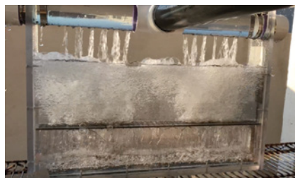
FIGURE 8. Tests were conducted with a 20% open area PIP, 4 in. above the parting box floor [72]. The liquid level at the bottom of the box was only about 1 in., with an air gap occupying the other 3 in. between the PIP and the floor of the box (Reprinted courtesy of AIChE)
